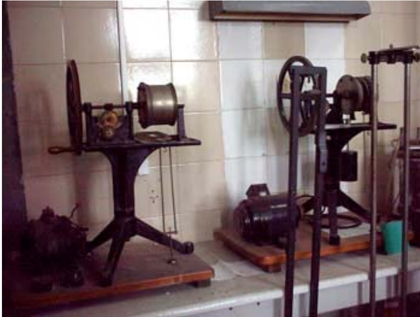
Fig. 6.6 – On the left an instrument to determine the mechanical equivalent of the calorie, acquired in 1930 from the famous German instrument maker Max Kohl by the Faculty of Sciences, University of Porto. On the right (behind another instrument) an exact 1:1 replica made in the workshop of the Department of Physics by an in-house technician. Both instruments are today part of the collection of the Museum of Science, Faculty of Sciences, University of Porto (original Inv. No. 1138/1929 and replica Inv. No. 2727/1962) (photo reproduced with the kind permission of the Museum of Science).
