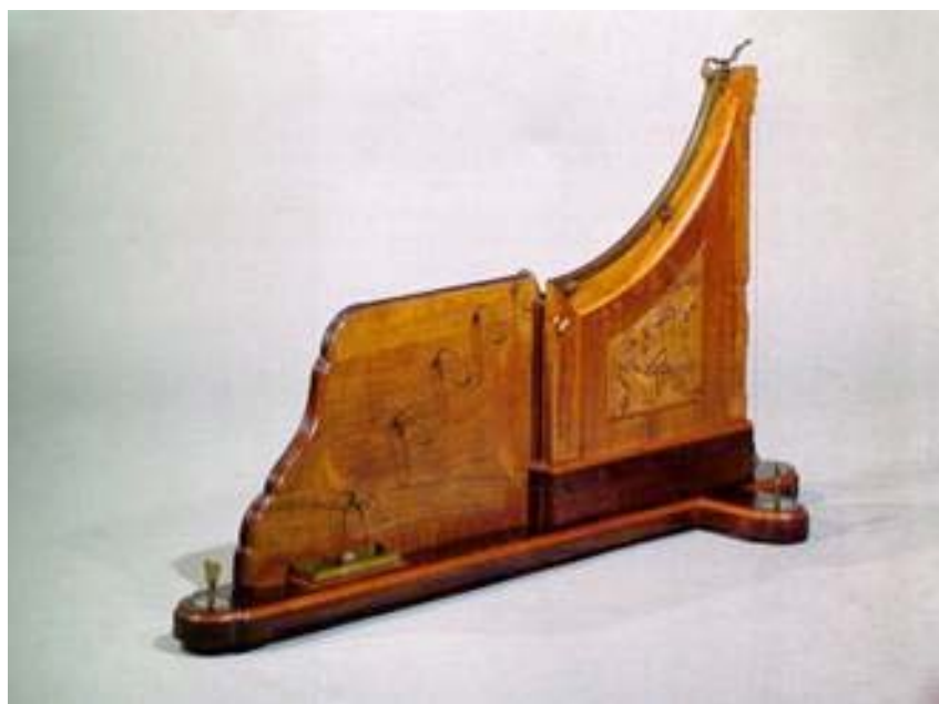
Fig. 4.7 – Device to illustrate the parabolic trajectory of projectiles, 18 th century cabinet of physics of the University of Coimbra ( Index 1788: G.IV.178) (photo José Pessoa © Divisão de Documentação Fotográfica do Instituto Português de Museus, reproduced with kind permission of the Museum of Physics, University of Coimbra).
