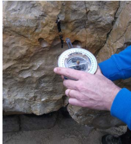
(b) Orientation of the sample: declination and inclination .
