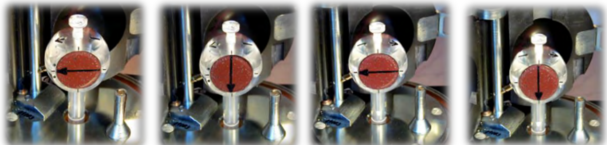
Figure 19. Different positions of the specimens of SPINNER MAGNETOMETER JR6/JR6A User's Manual AGICO.
